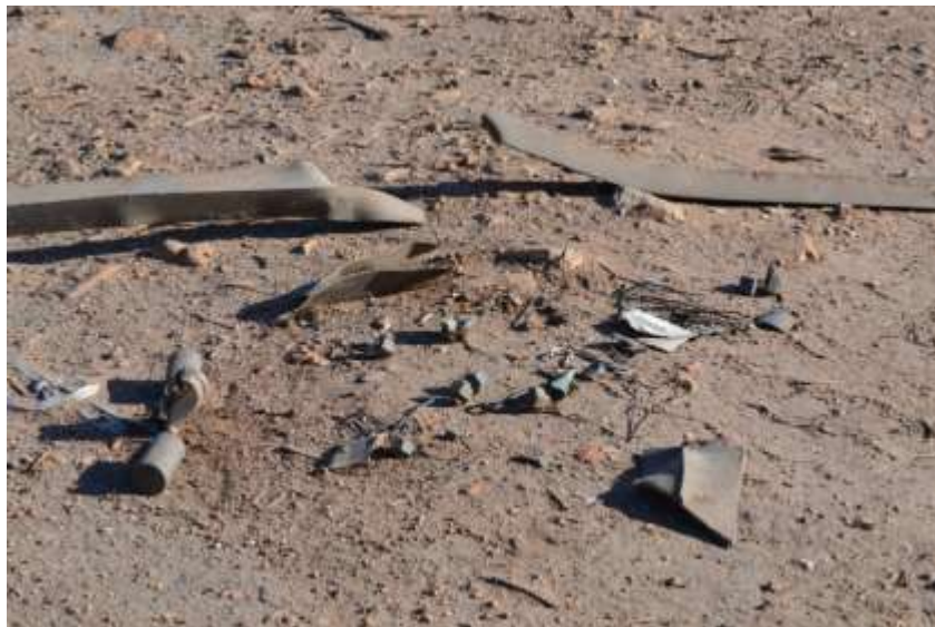
Figure 3: Tower debris found at the Aliso HAY in May 2013 by the CPUC EM. The trash was reported to SCE at the time and clean up did occur; however, debris is still being found at this location.
