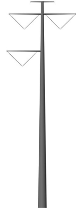
500-kV single-circuit TSP
