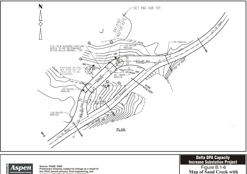
Figure B.1-6 Map of Sand Creek with Proposed Temporary Bridge
