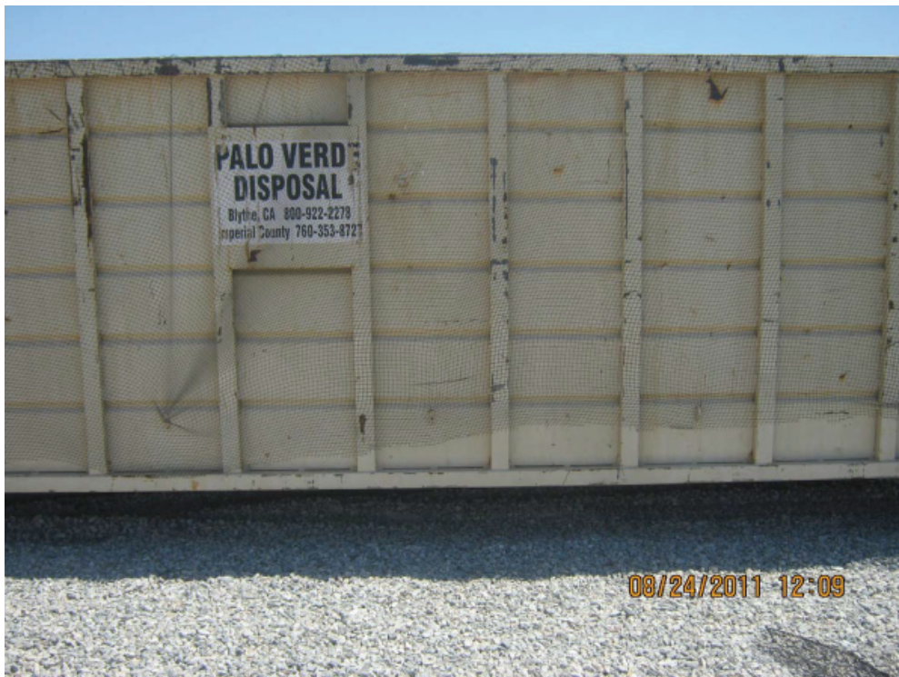
Figure 8: Netted roll-off bins onsite at DC1 and DC2 Construction Yards.
