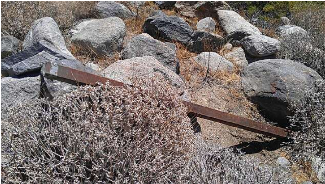
Figure 5. Micropile drill deck leg that dislodged and fell from the helicopter during transport from Tower 1032 to HLZ H2 (Photo courtesy of FRED).
