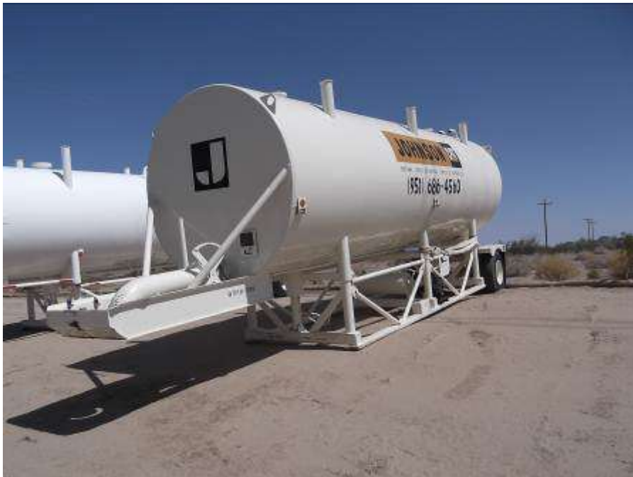
Figure 6. Water stand tanks staged at Tower 2443ALT with no secondary containment.
