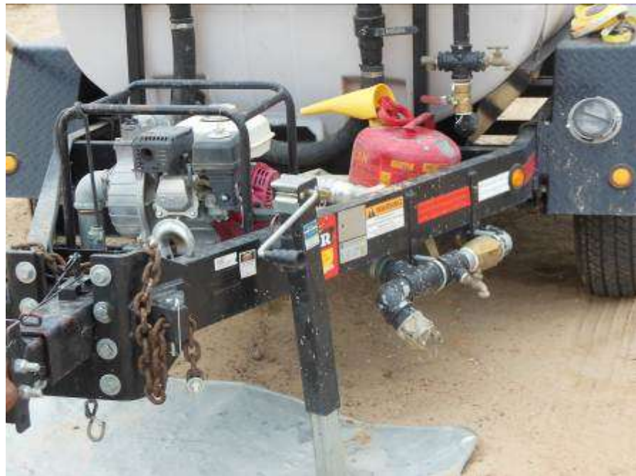
Figure 8. Gasoline can with no secondary containment at Tower 2637.
