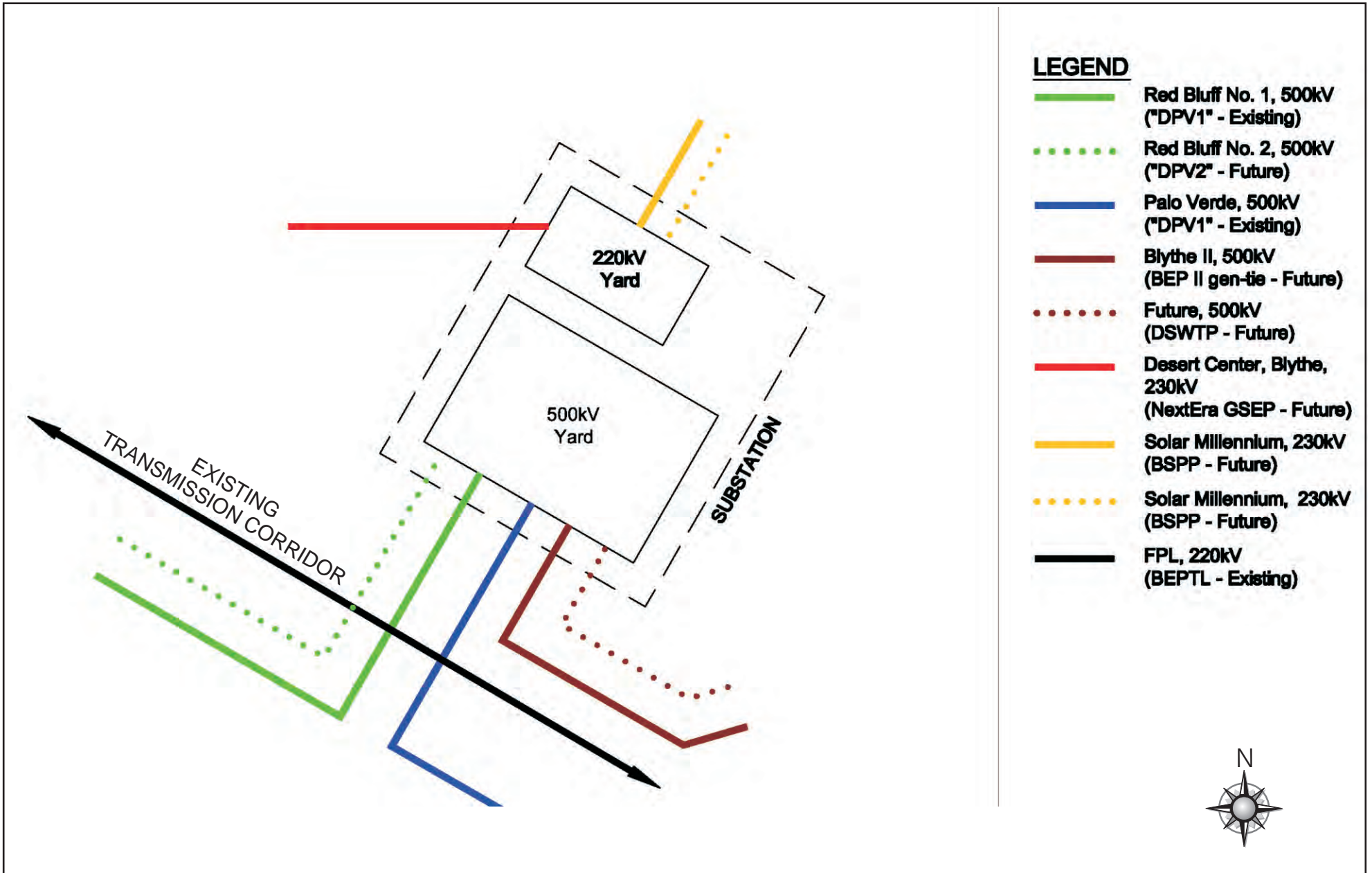
Figure Ap.1-3B Avoidance Alternatives Substation Configuration (Perpendicular Orientation)
