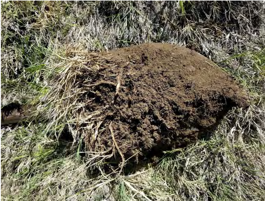
Photograph 9: Feature ID 2008. Soil pit number two. Photo shows unsaturated soil without stratified layers.
