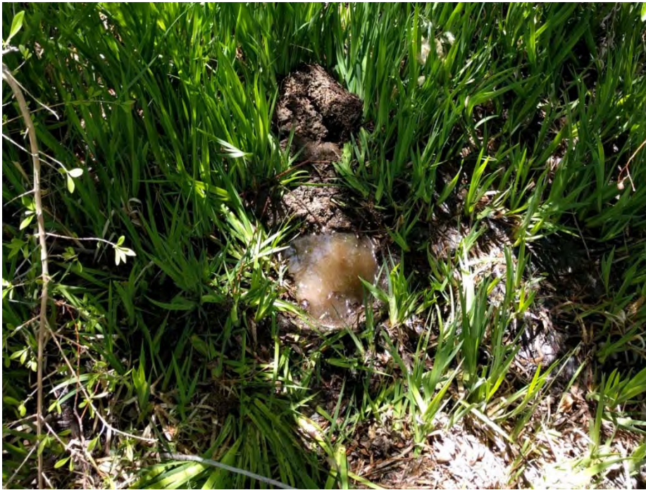
Photograph 1: Feature ID 2008. Soil pit number one. Photo shows water table just below surface of soil sample.
