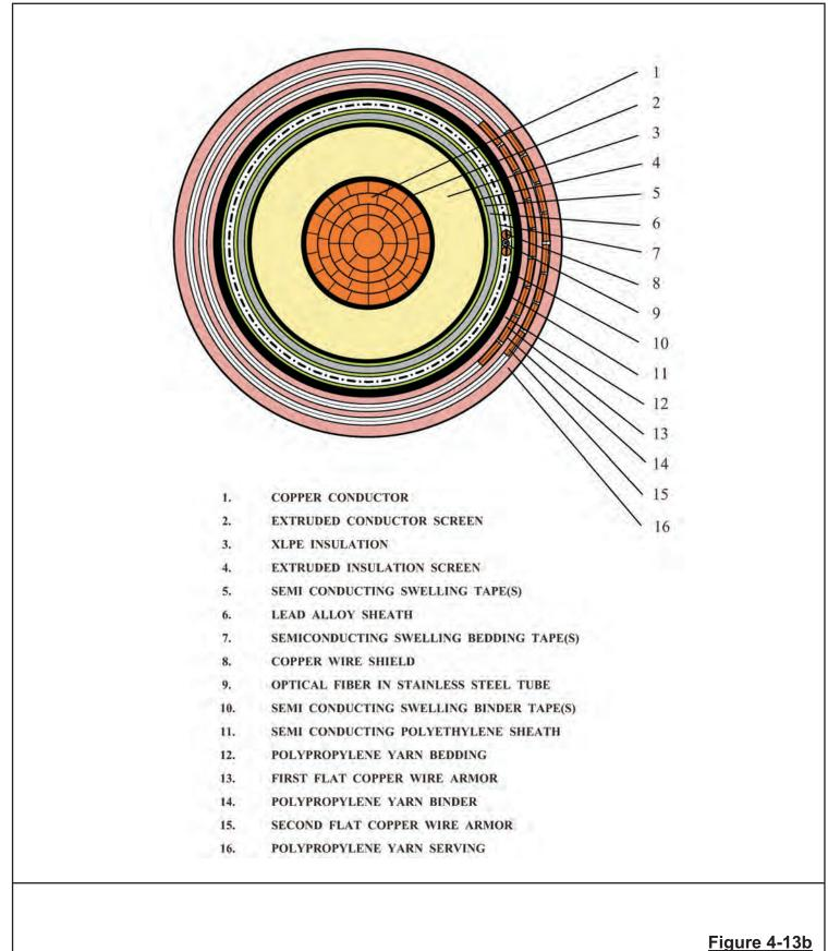
Aspen wironmental Group Cross Section of the Proposed 230 kV XLPE Submarine Cable with Double Copper Armoring Design
