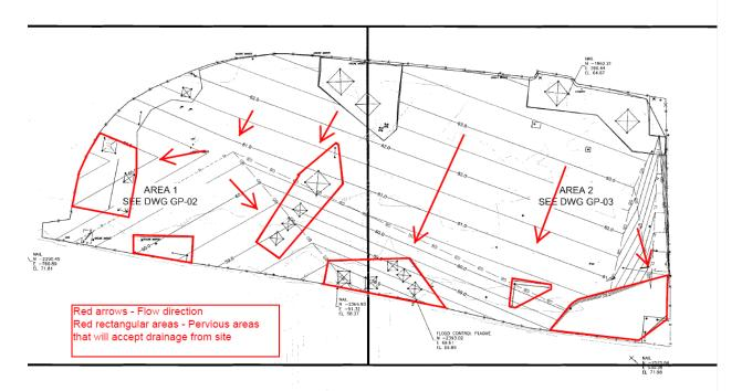
GRADING PLAN AND DRAINAGE FLOW DIRECTION
