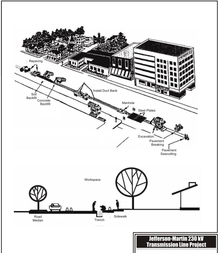
Figure B-12a **Typical Underground Construction Process** within Roadways
