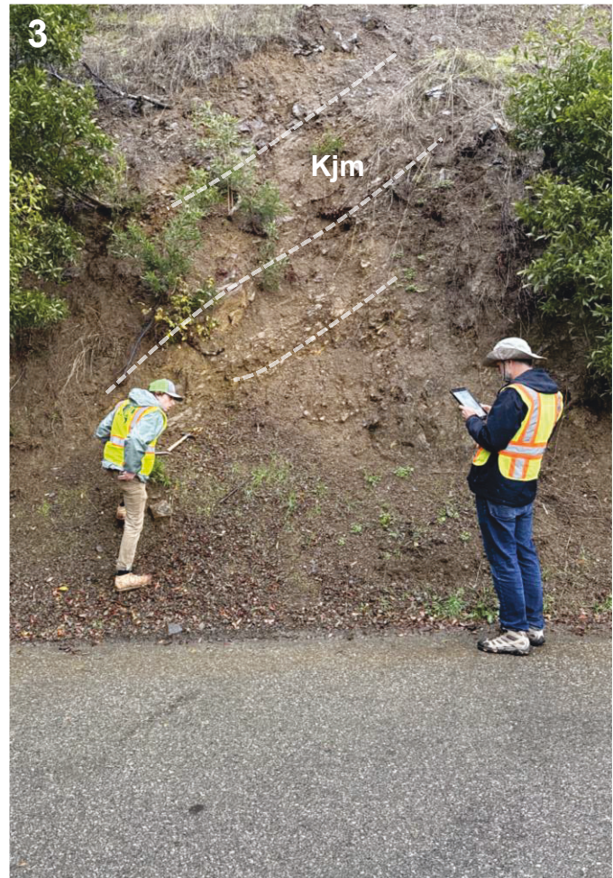
Photo 2: Field Locality 6 – Jurassic diabase/ basalt or graywacke (Jsv/ Jb) with planar, secondary felsic mineralization; Photo 3: Field Locality 7 – dipping beds in the Cretaceous unit (Kjm) directly northeast of linear drainage.
