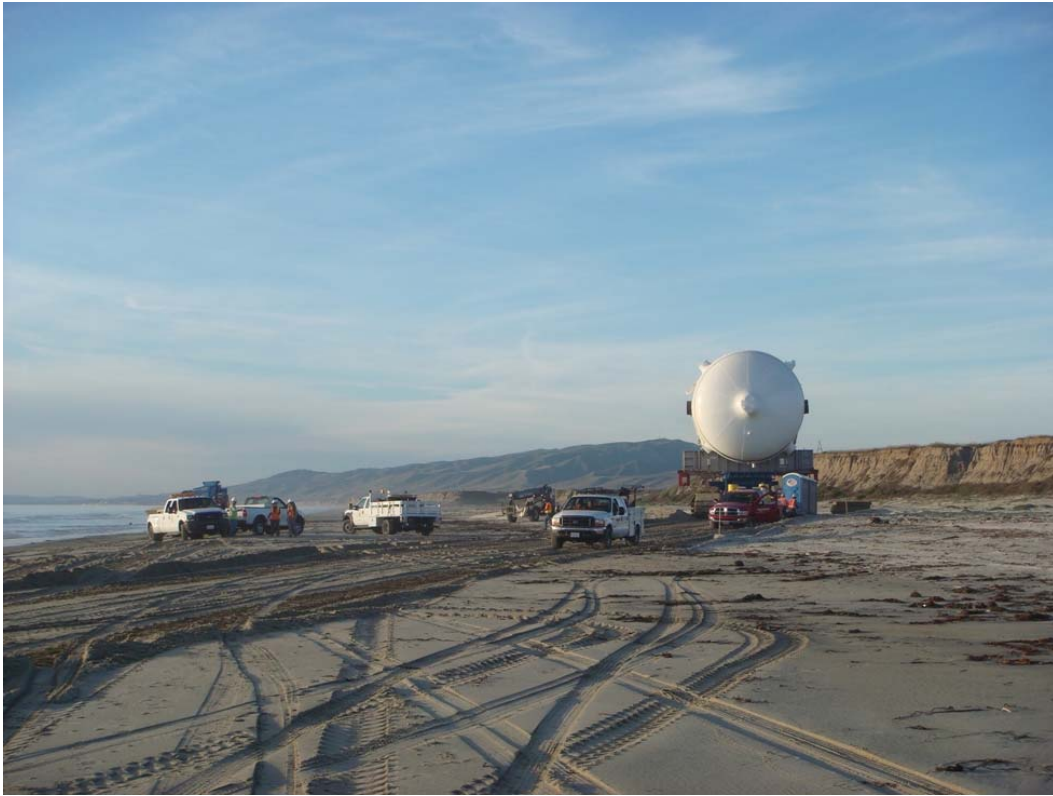
Figure 3: The RSG at a layover area above the mean high tide line along the beach route. The RSG was staged overnight in the layover areas and resumed transport during the next low tide.
