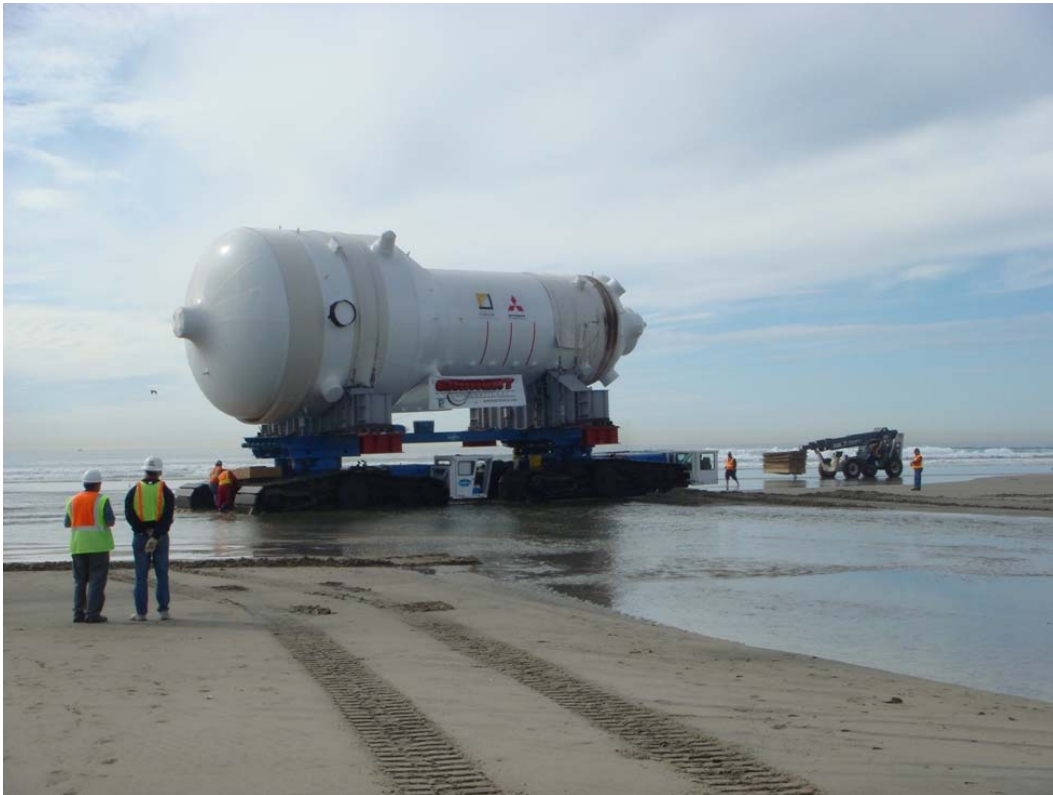
Figure 1: RSG on the crawler crossing the Santa Margarita River along the beach route on MCBCP.
