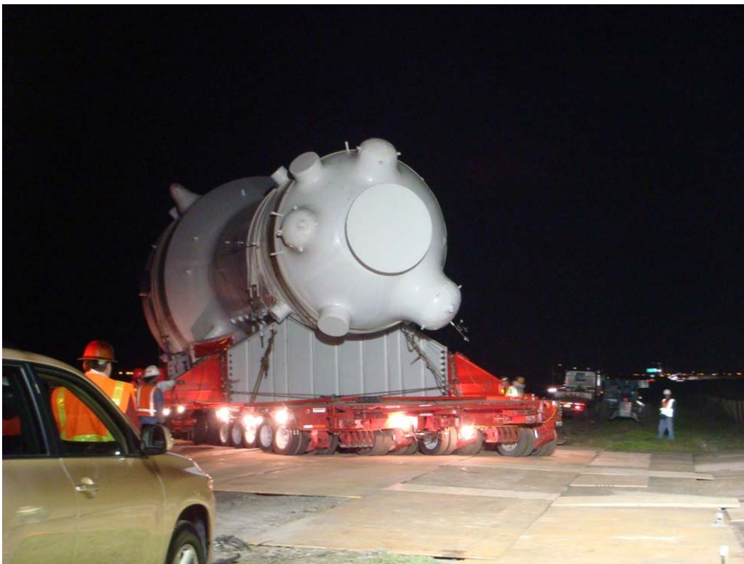
Figure 4: RSG transport along Interstate 5 on the Goldhofer. Steel plates were used to protect curbs and pavement.
