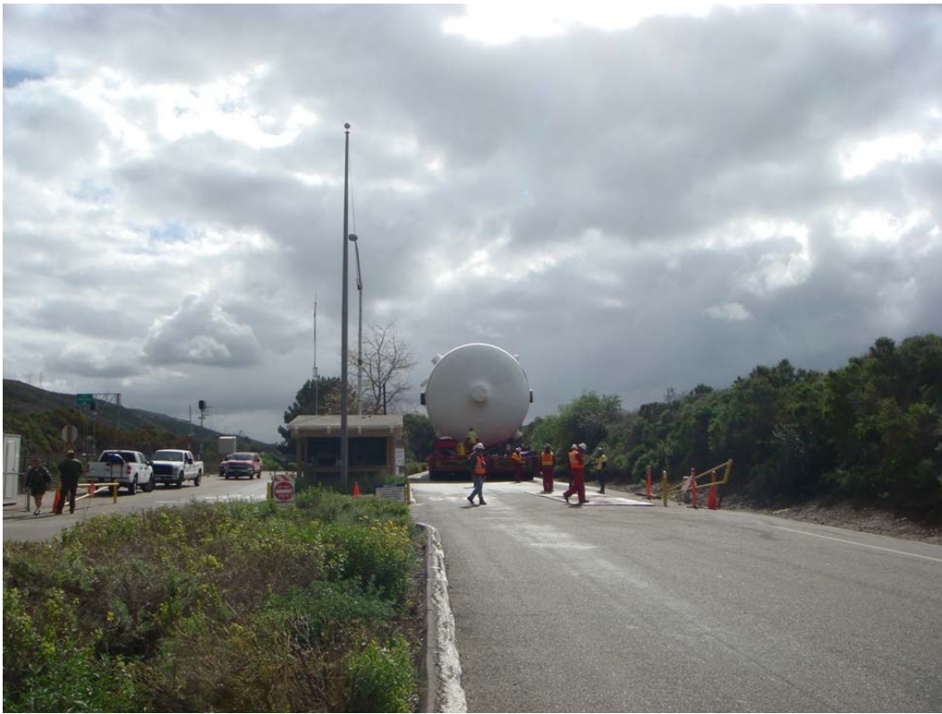
Figure 5: Transport of the RSG on the Goldhofer through San Onofre State Park.
