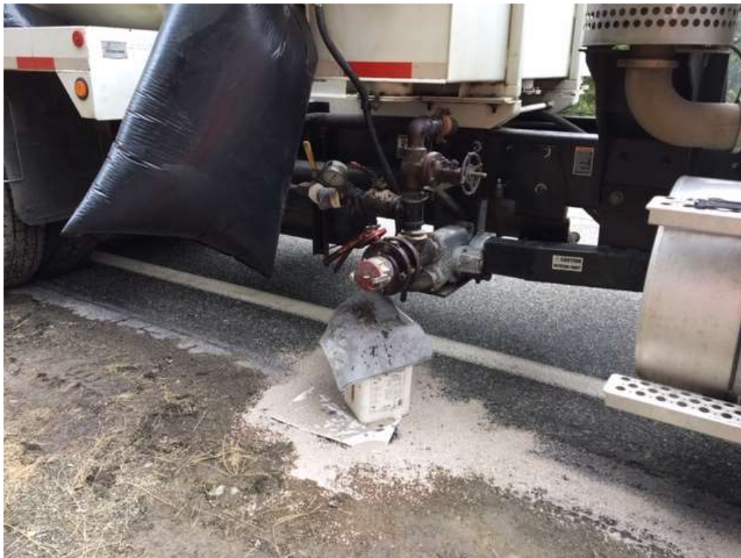
Figure 2 – Small leak on vac-truck at MP 24.5 clean-up – May 22, 2019.
