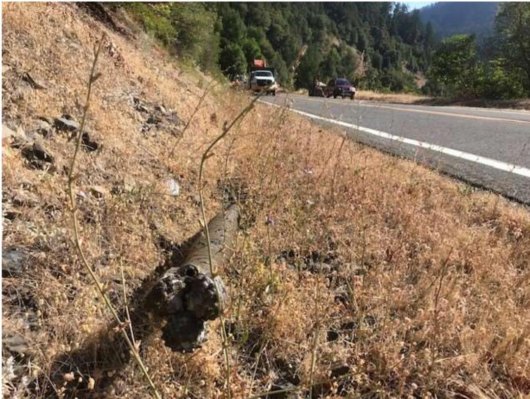
Figure 3 – End of drill-bit “popped-out” at MP 20.64, view south, August 7, 2019.
