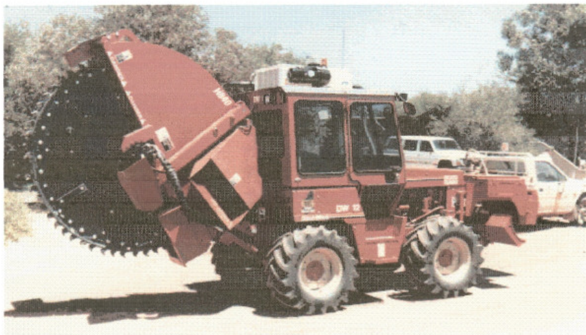
Continuous trenching equipment used to install underground power lines in Australia
