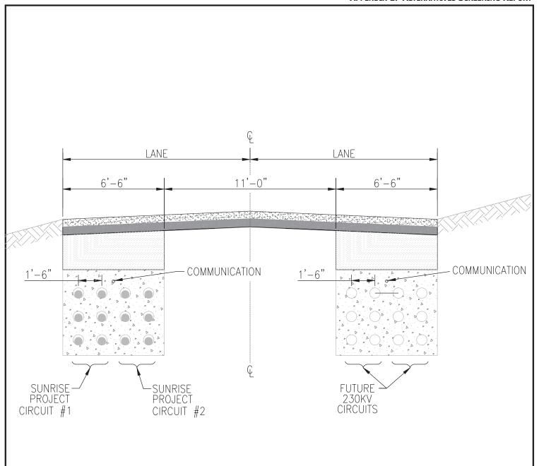
This configuration would apply only where the road is narrow with no shoulder. Future Phase circuits are shown in addition to Proposed Project circuits. Duct banks are shown for two cables/ph.
