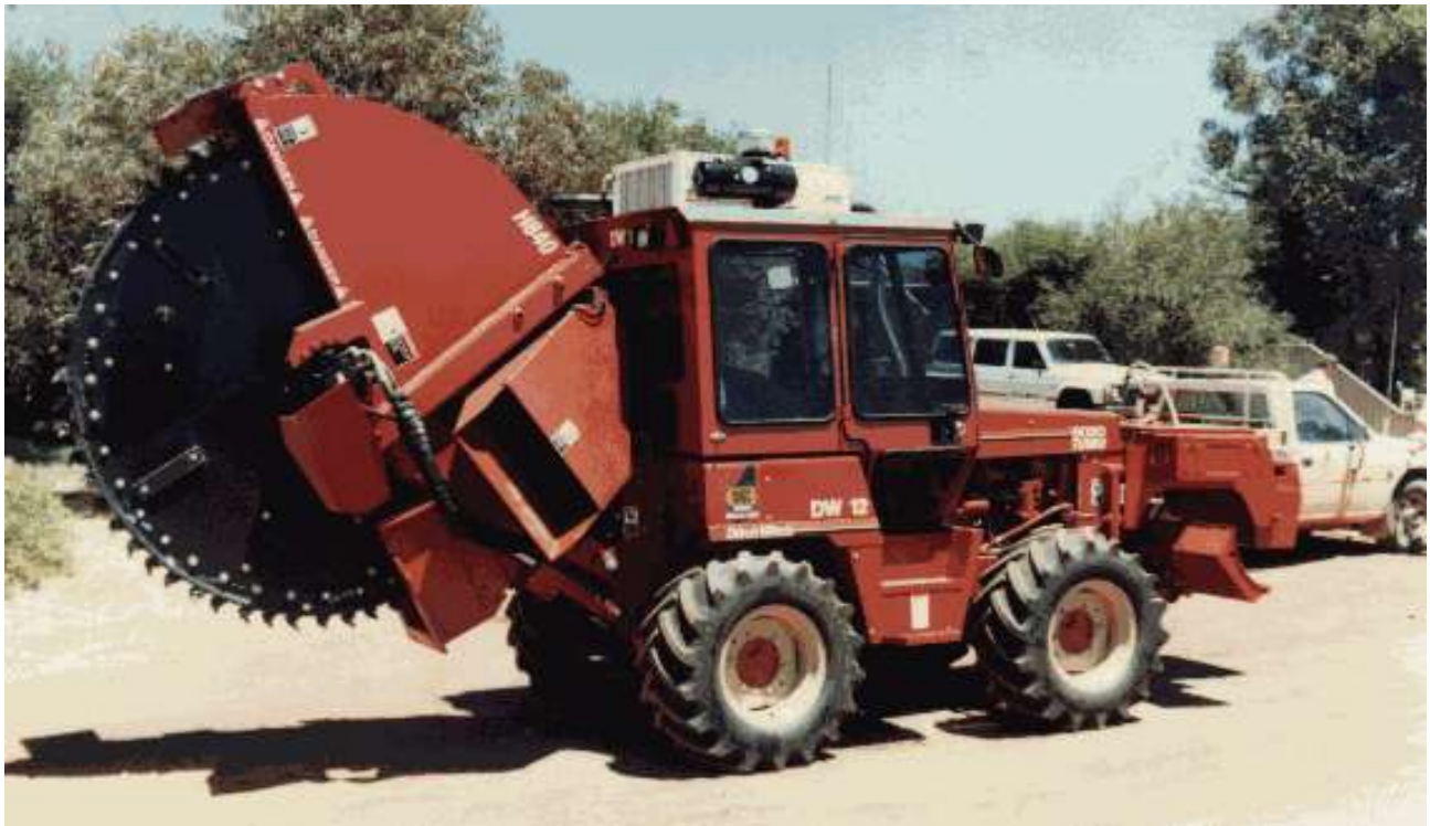
Continuous trenching equipment can slice through decomposed granite soils of Imperial and eastern San Diego County
