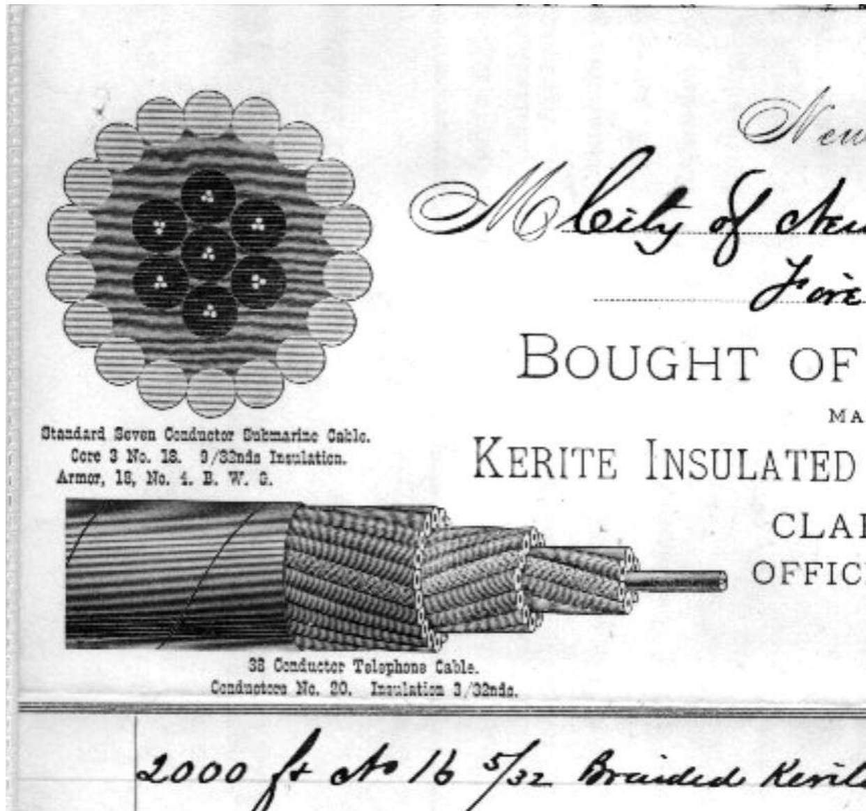
Construction detail of a 7 conductor submarine power cable and a 38 conductor telephone cable during the 1880's
