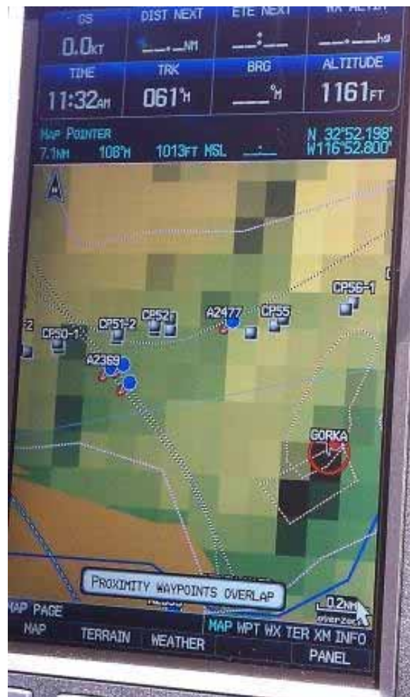
Figure 10: GPS unit display in helicopter showing tracks to Helix Construction Yard and avoidance of sensitive land owner property. (Link 5)
