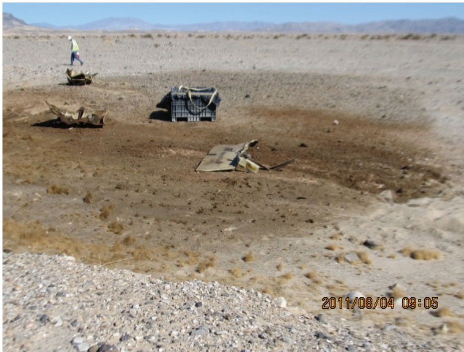
Figure 5: Diesel fuel spill resulting from a dropped compressor unit, Link 1. (Photo courtesy of Andrew McGann and David Mendez.)
