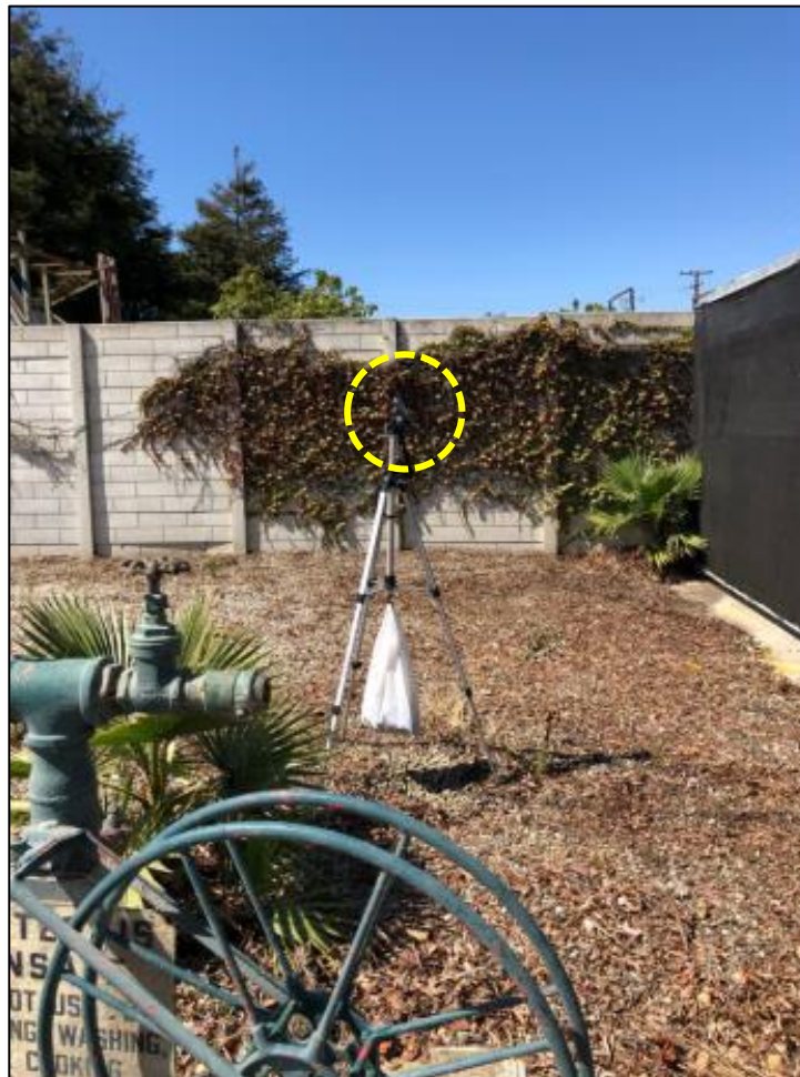
Exhibit M-5.1 – Sample photograph, looking north, of the deployed sound level meter (encircled with yellow dashes) at the northern monitoring location (NML) onsite near the Ventura Compressor Station (VCS) access gate during the June 2021 field survey
