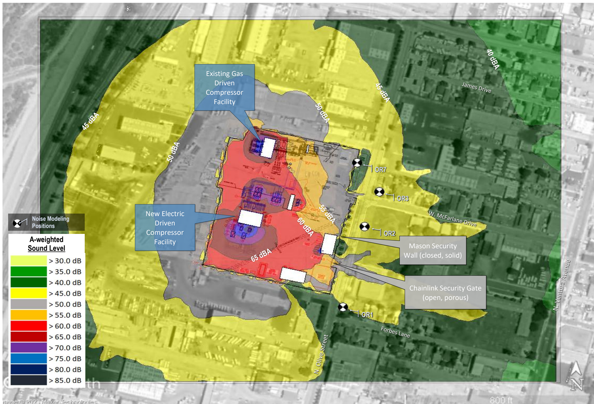
FIGURE 3 Predicted Supplemental EDC Alternative Operation: Two Electric-Driven and Three Engine-Driven Compressors
