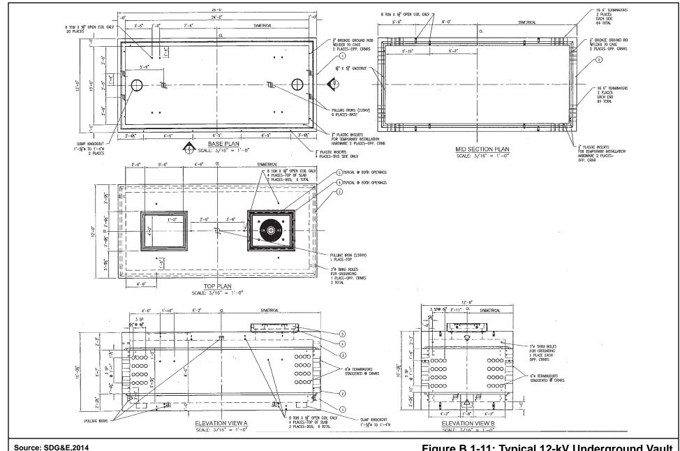
Figure B.1-11: Typical 12-kV Underground Vault
