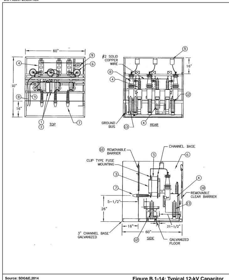
Figure B.1-14: Typical 12-kV Capacitor
