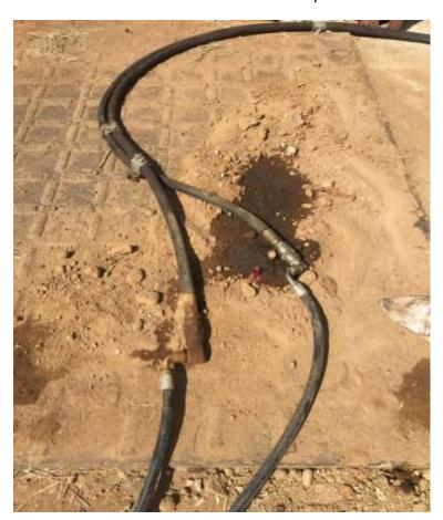
Figure 6 – Same hydraulic leak observed the morning of May 18 after crews had used dirt to contain and soak up the spill.
