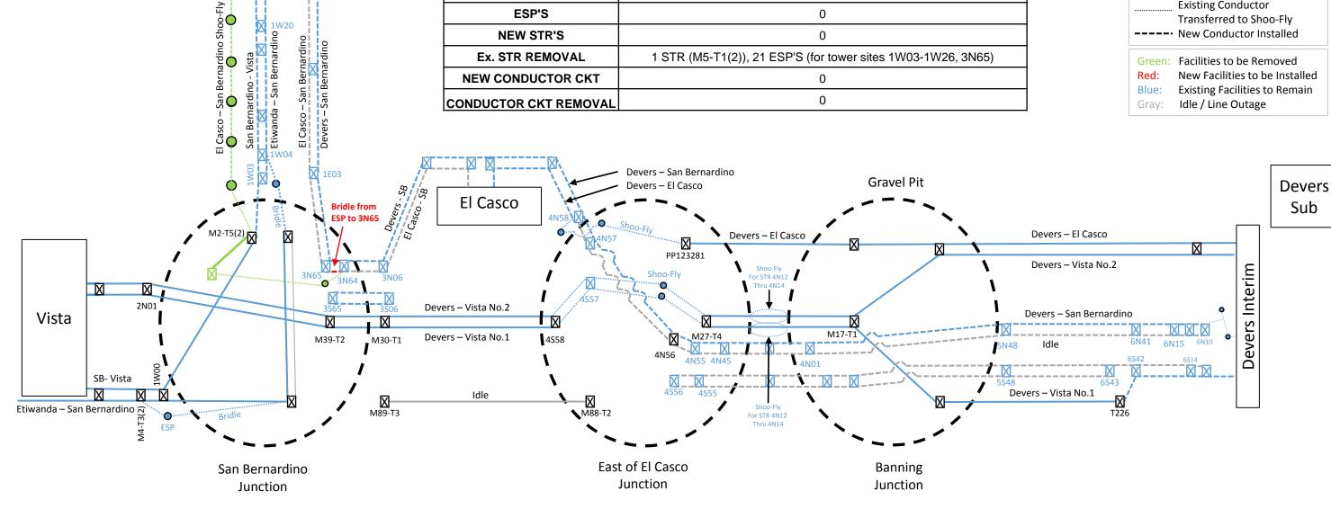
Move 8 transfers the El Casco – San Bernardino circuit from the shoo-flies in Segment 1 to the new East structures in Segment 1 and completes the construction of this circuit. Following the tie in of the EC – SB circuit at 3N65 the shoo-flies in Segment 1 can be remove and construction within the residential portions of Segment 1 will be complete.
