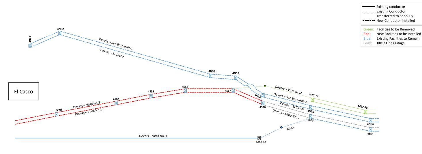
Following the transfer of the Devers – Vista #2 to its proposed location on the new structures all remaining structures (including shooflies) East from the East of El Casco Junction will be removed non-outage.
