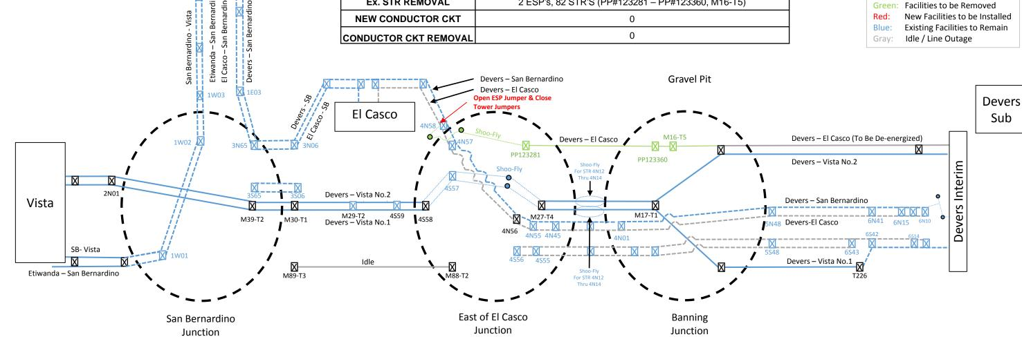
Move 11 will transfer the Devers – El Casco circuit from the existing structures and shoo-flies to the new structures and conductor by re-positioning the jumpers at structure 4N58. Following this minimal scope the D-EC circuit will be complete. The represented removal scope can be completed non-outage following the re-positioning of the jumpers.
