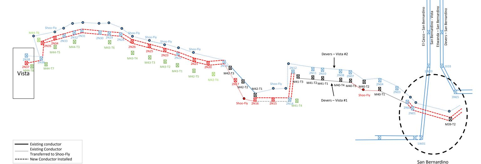
Where the previous move shoo-flied the Devers – Vista #2 structures the existing structures will be removed and the new structures will
