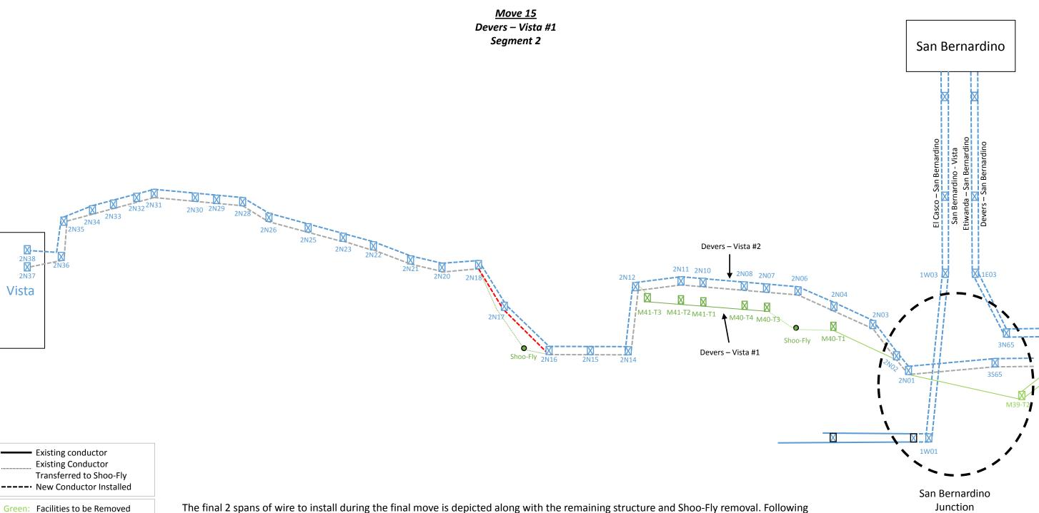
The final 2 spans of wire to install during the final move is depicted along with the remaining structure and Shoo-Fly removal. Following this move the West of Devers Upgrade Project is complete.
