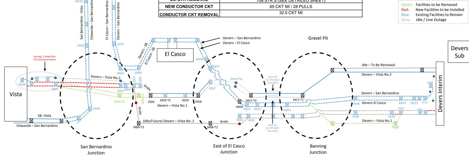
Move 13 will conductor the Devers – Vista circuits over through the San Bernardino Junction (SB-V and E-SB circuits will be guarded now that they are accessible in their new location). Also sections of Segment 2 will be replaced with new structures and strung with new conductor. Behind El Casco substation the Devers – Vista #2 will utilize the previous Devers - San Bernardino structures as a shoo-fly preparing for the construction of the new towers in this location.
