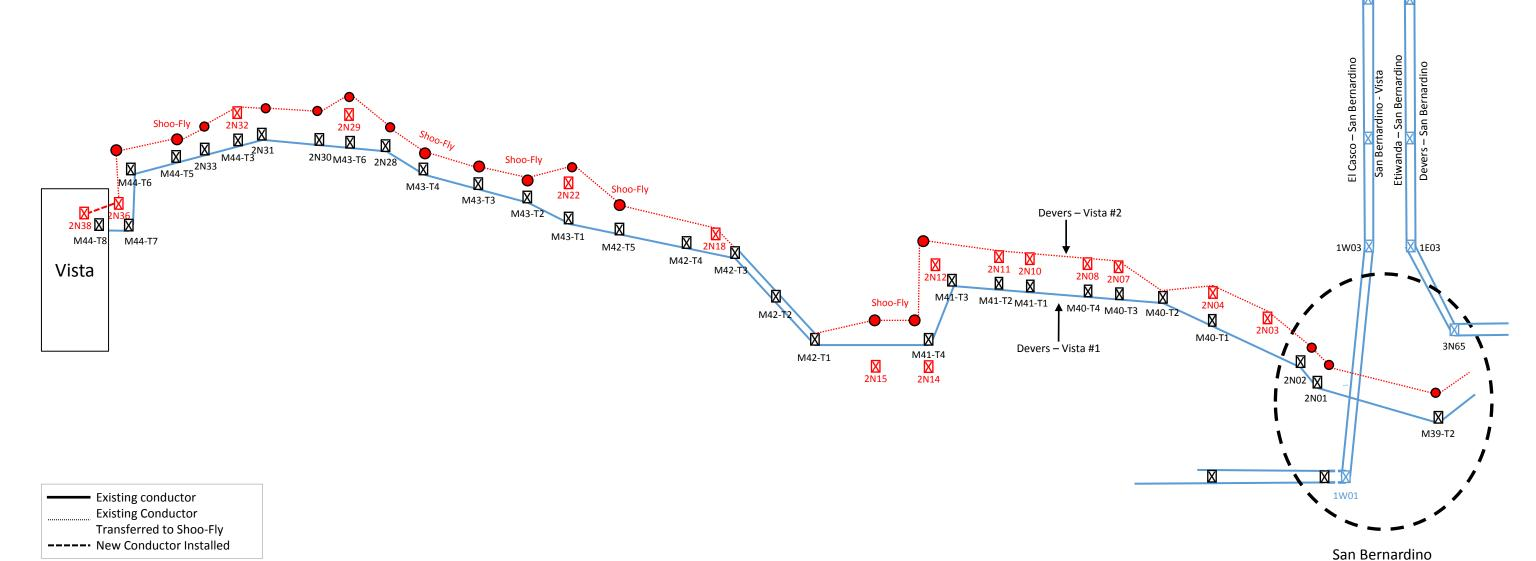
New structures installed in this move will act as shoo-flies to isolate the existing structures and where the new structures cannot be installed (due to conflicts with the existing towers) shoo-flies will be installed to isolate the structure locations setting up for removal and construction of new structures under a single line outage.
