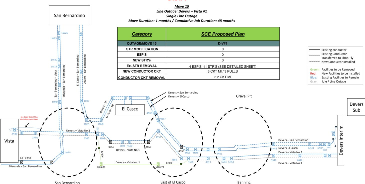
Move 15 completes the West of Devers Upgrade following its 2 span wire installation in Segment 2 and the re-positioning of conductor behind El Casco Substation. Removal of the Devers – Vista Shoo-Fly can be completed non outage once spans at either end have been put into their final proposed locations.
