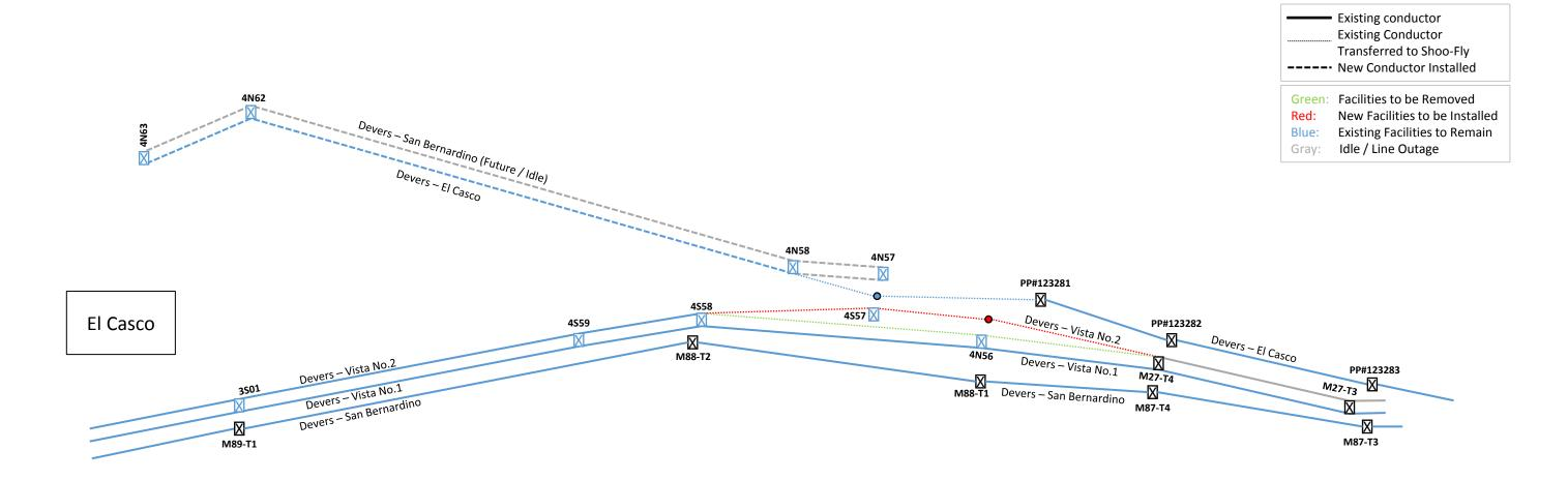
This detail represents the Devers – Vista #2 circuit being transferred from the North position of the 4N56 structure to the new 4S57 (installed in previous move) and also to a shoo-fly structure at 4N56 opening up the North position on 4N56 for its future circuits (this position will ultimately be occupied by the D-SB circuit in the final configuration).
