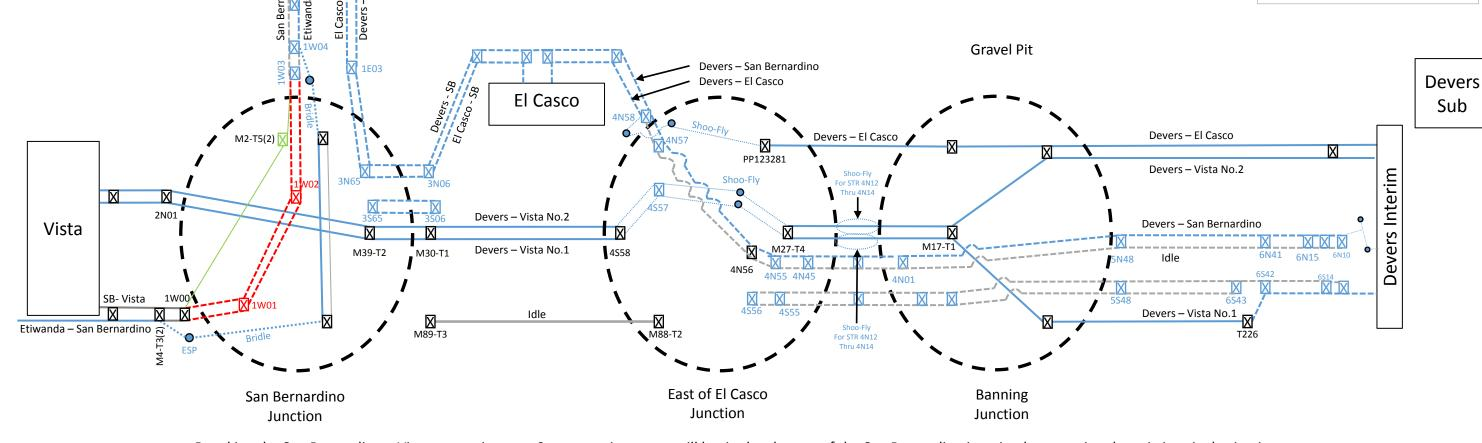
By taking the San Bernardino – Vista outage in move 9 construction crews will begin the cleanup of the San Bernardino junction by removing the existing single circuit towers and installing two (2) new double circuit structures and stringing the respective conductor. Following this move the remainder of the East towers in Segment 1 will be complete and the San Bernardino – Vista circuit will be also be completed as a result.
