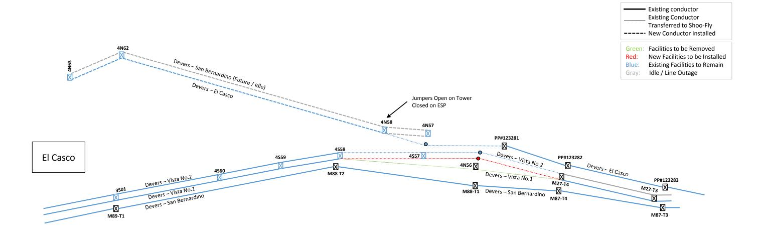
This detail represents the Devers – Vista #1 circuit being transferred from the South position of the 4N56 structure to the new 4S57 (installed in previous move) and also to a shoo-fly structure at 4N56 opening up the South position on 4N56 for its future circuits (this position will ultimately be occupied by the D-EC circuit in the final configuration).
