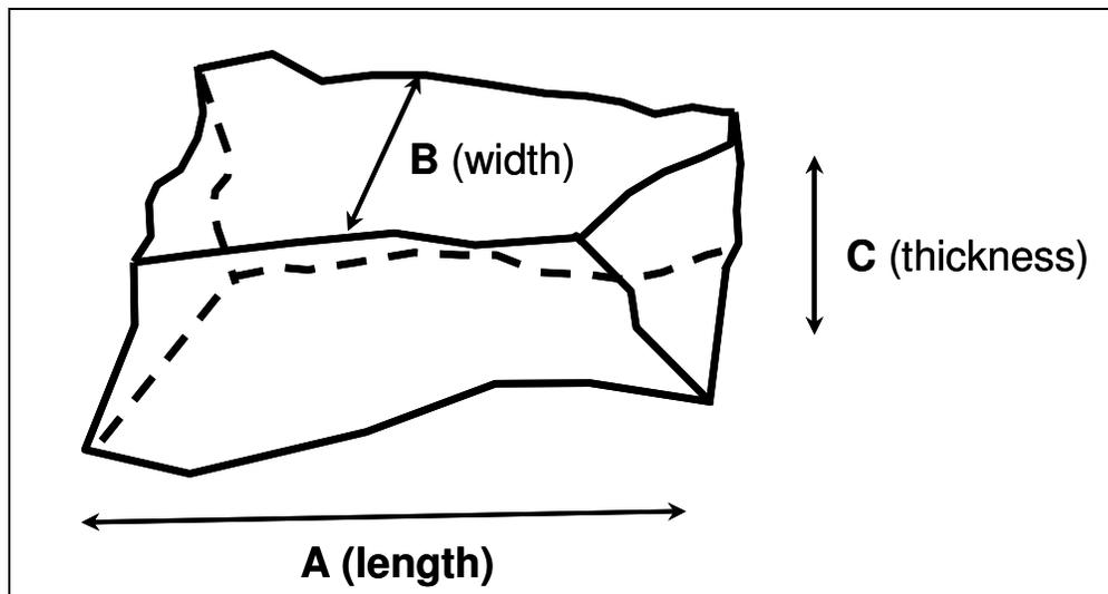
Figure 4.1. Riprap shape described by three axes.
