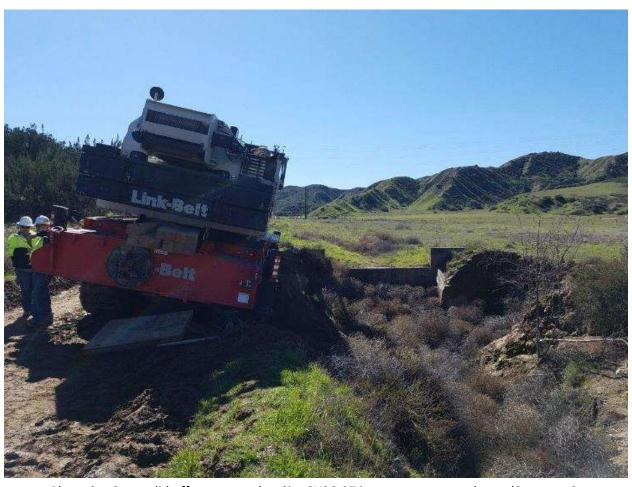
Photo 3 – Crane slid off access road to Site 3X06-07 into an unapproved area (Segment 3; February 11, 2019) (photo courtesy of SCE).
