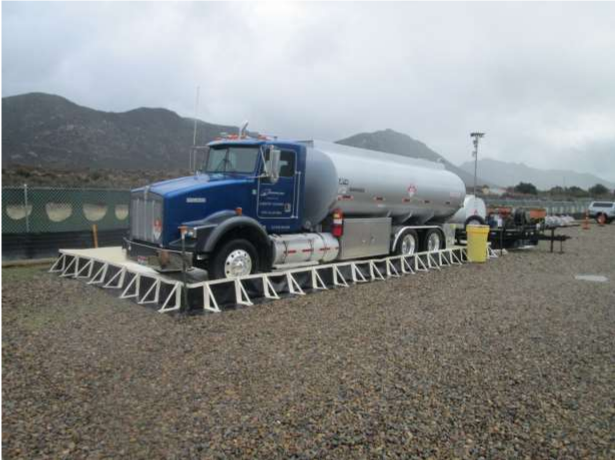
Photo 5: In accordance with the project SWPPP, secondary containment was observed being utilized beneath a jet fuel storage tank at Anderson Staging Yard (TL 629E).
