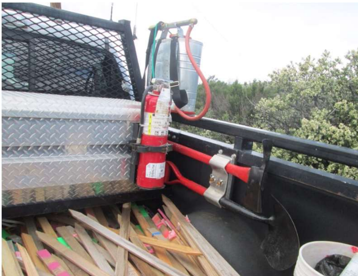
Photo 2: Pickup trucks used along the ROW were equipped with a 5 gallon backpack pump, Pulaski, round point shovel, and 2A10BC fire extinguisher in accordance with the CFPPP and MM-FF-1. Biological monitors were observed present during staking in accordance with MM BIO-23.
