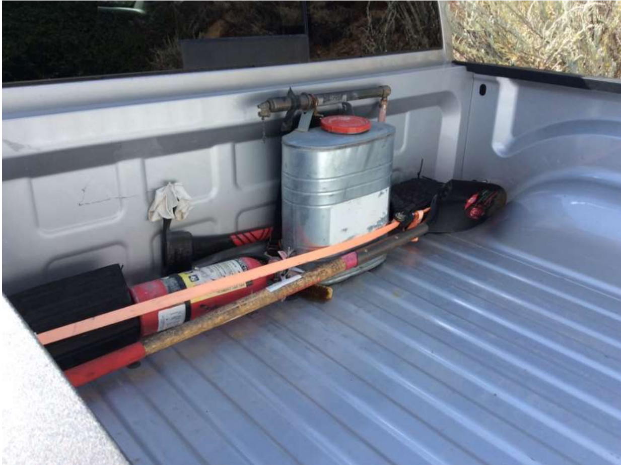
Photo 5: During observations along TL 682, project vehicles were equipped with a 5-gallon backpack pump, a Pulaski, a round point shovel, and a 2A:10B:C fire extinguisher in accordance with the Fire Prevention Plan (MM FF-1).
