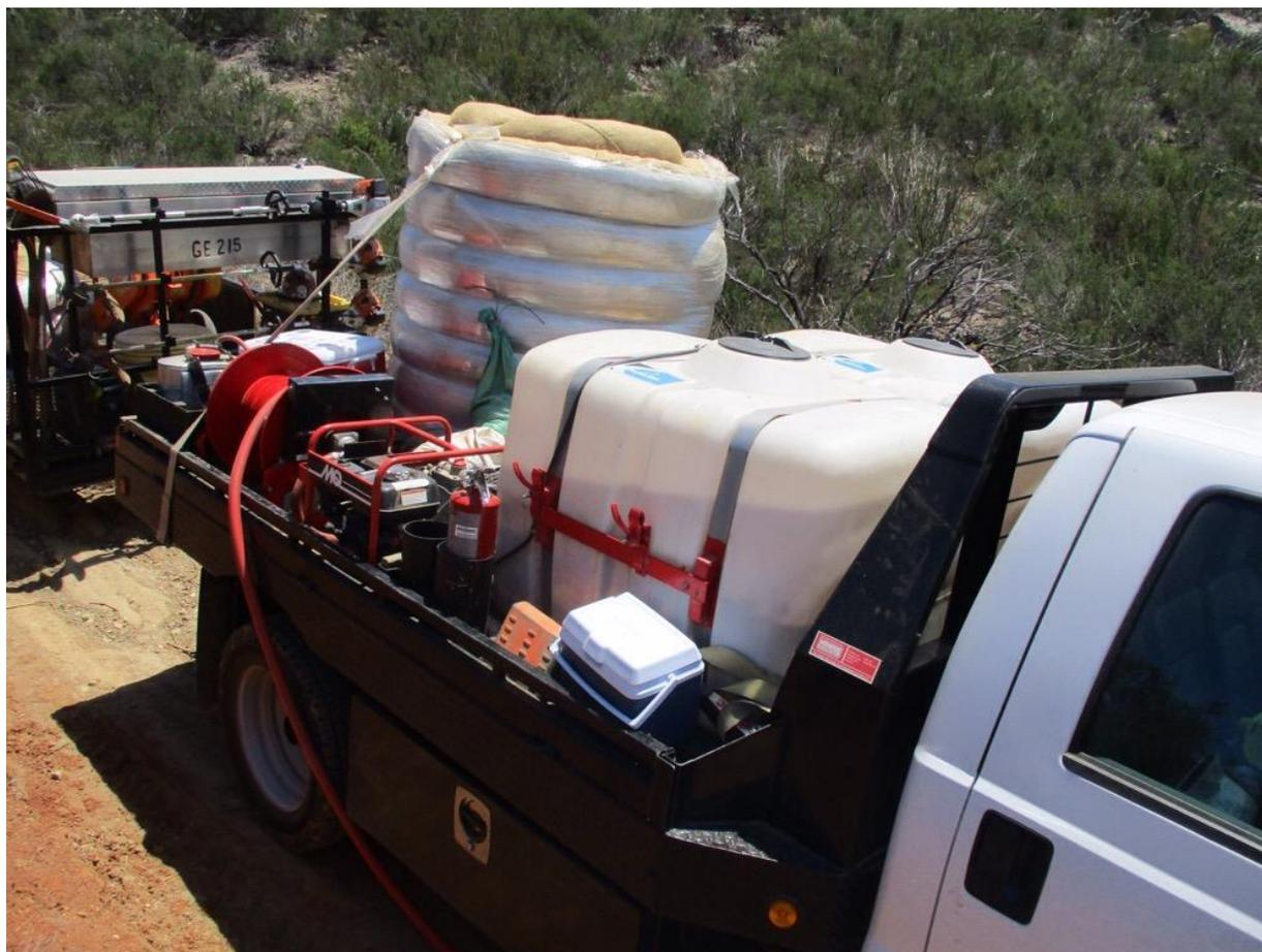
**Photo 4:** In addition to a 5 gallon backpack pump, round point shovel, Pulaski, and 2A10BC fire extinguisher, the vegetation clearing crew at Z571449 (TL6957) was equipped with 100 gallons of water with a pump and hose (as required for chipping) and a crew member was observed wetting down the area during chipping in accordance with the CFPPP fire prevention matrix (on CNF land).
