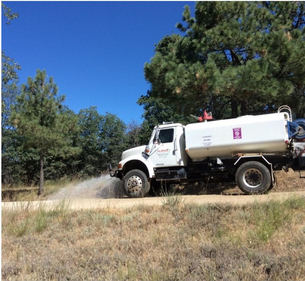
**Photo 1:** A water tender was observed applying water on Los Huecos Road (C 440 Phase II) to minimize dust emissions throughout the day in accordance with APM AIR-02.
