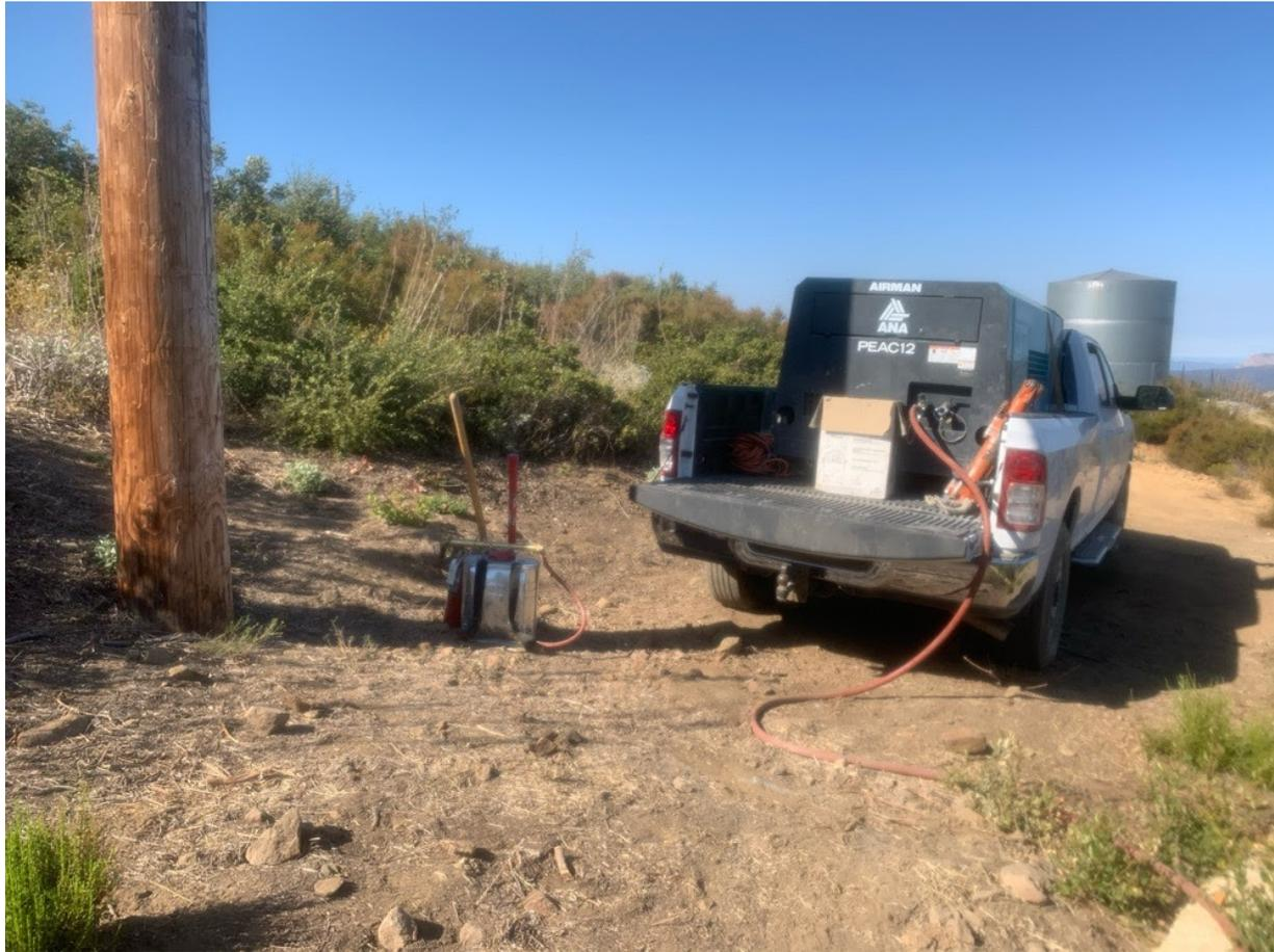
**Photo 4:** A running air compressor at Pole P258572 (C 79B) had at least 5 feet of clearance from combustible material on all sides and a full set of fire tools (5-gallon backpack pump, round point shovel, Pulaski, and 2A10BC fire extinguisher) within 50 feet in accordance with the CFPPP Fire Prevention Matrix for combustion engine use off USFS land with an Elevated FPI.
