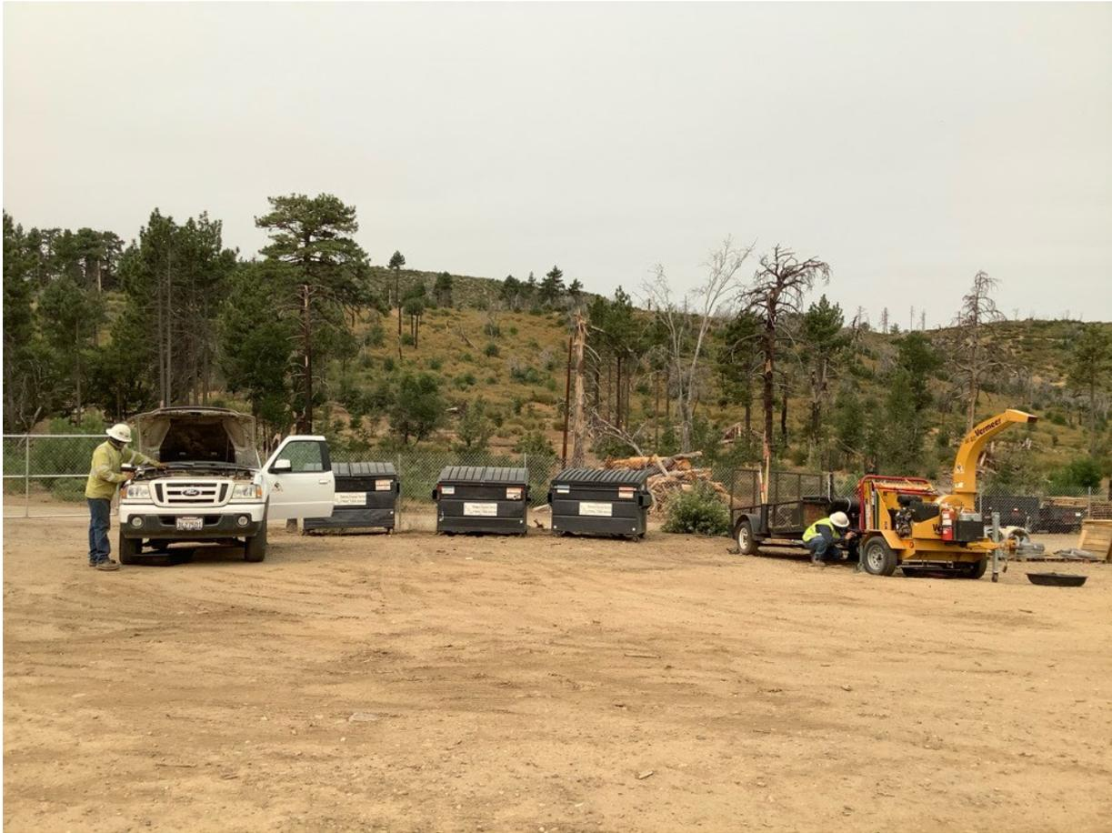
**Photo 5:** A crew was observed conducting vehicle and equipment maintenance at Shrine Camp Staging Yard (C 440). Drip pans were observed under vehicles and equipment during maintenance to prevent leaks or spills from being discharged onto the ground in accordance with the SRNP and MM PHS-2.
