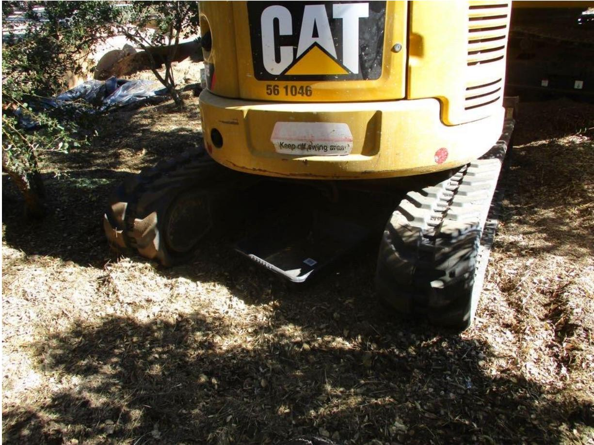
**Photo 5:** During pole hole drilling at Pole Z172739 (TL 629A), the crew was observed using a drip pan beneath staged equipment to prevent leaks or spills from being discharged into the soil in accordance with MM PHS-2.
