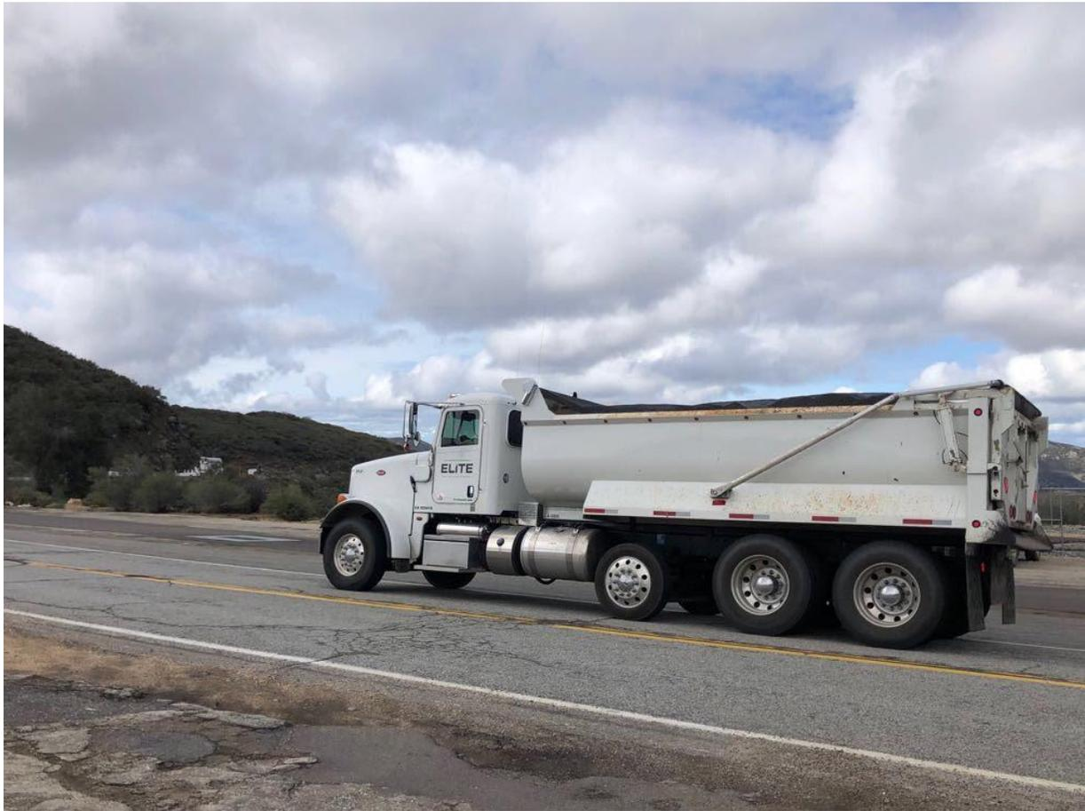
**Photo 3:** Haul trucks used for dirt export from C 440 were observed utilizing load covers to prevent dust emissions in accordance with APM AIR-02.
