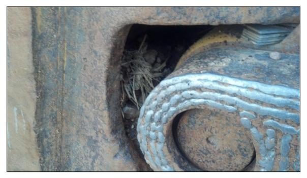
Photograph 2: Vegetative debris present in the tracks of the bulldozer.
