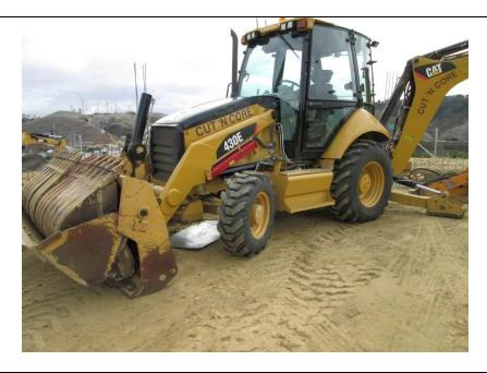
**Photo 4:** In accordance with APM-HYD-1, drip pans were used beneath staged construction equipment to prevent potential leaks from being discharged onto the soil.
