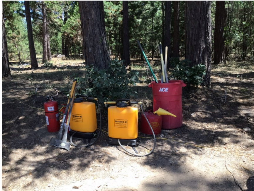
Photo 5: Fire suppression tools staged onsite in accordance with MM HAZ-2
