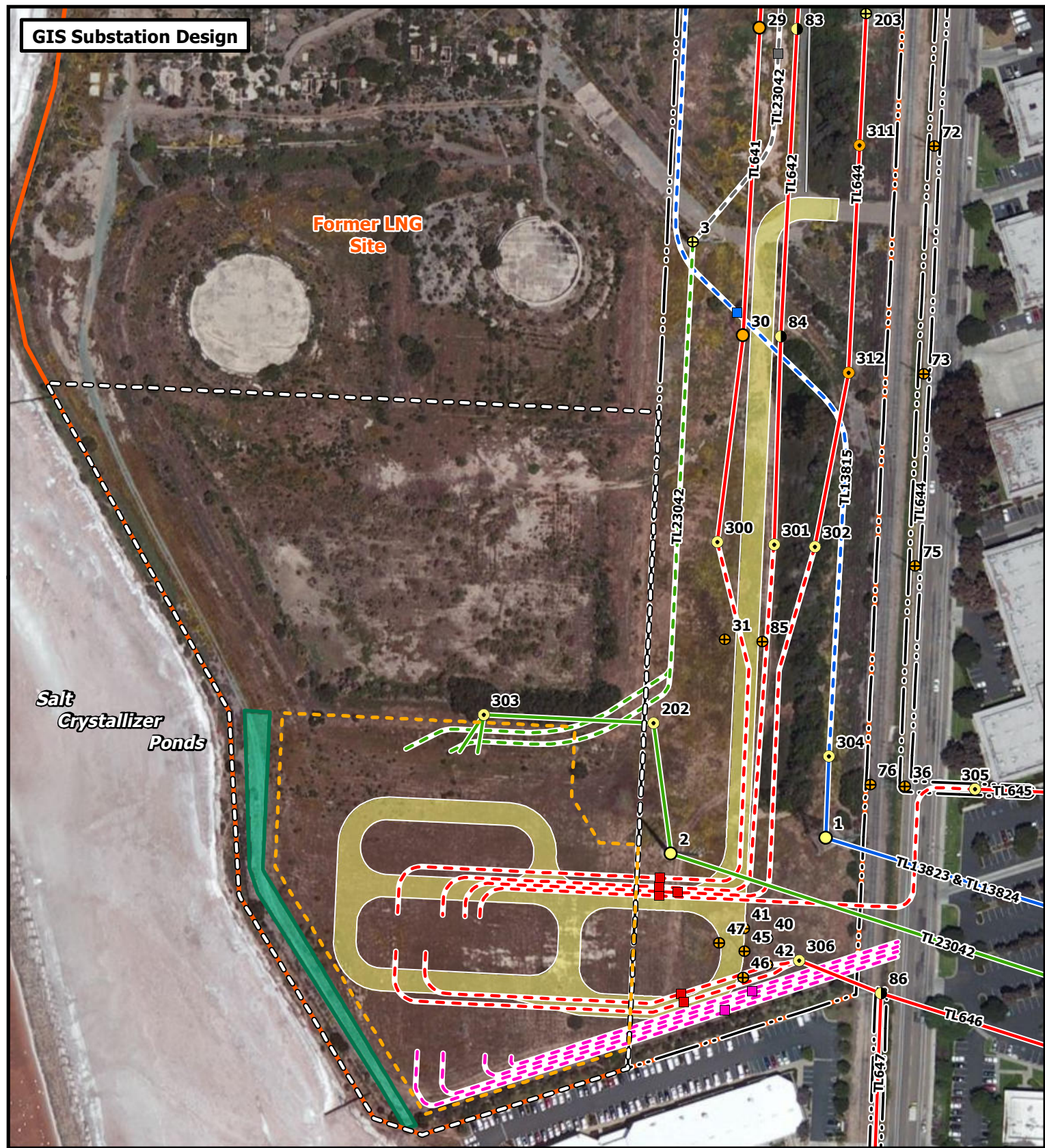
Figure 2: GIS Versus AIS Interconnection Comparison Map
