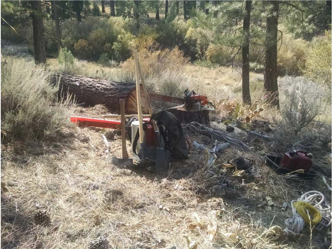
Photo 4: Firefighting equipment available within 25 feet of any chainsaw activity consistent with APM-HAZ-5.
