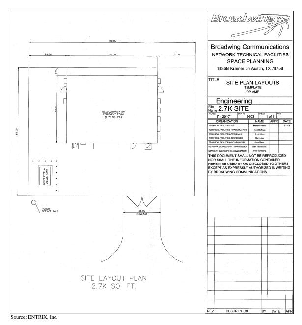
Figure 2.5-13. Typical Footprint for Regeneration Station Serving Multiple Customers
