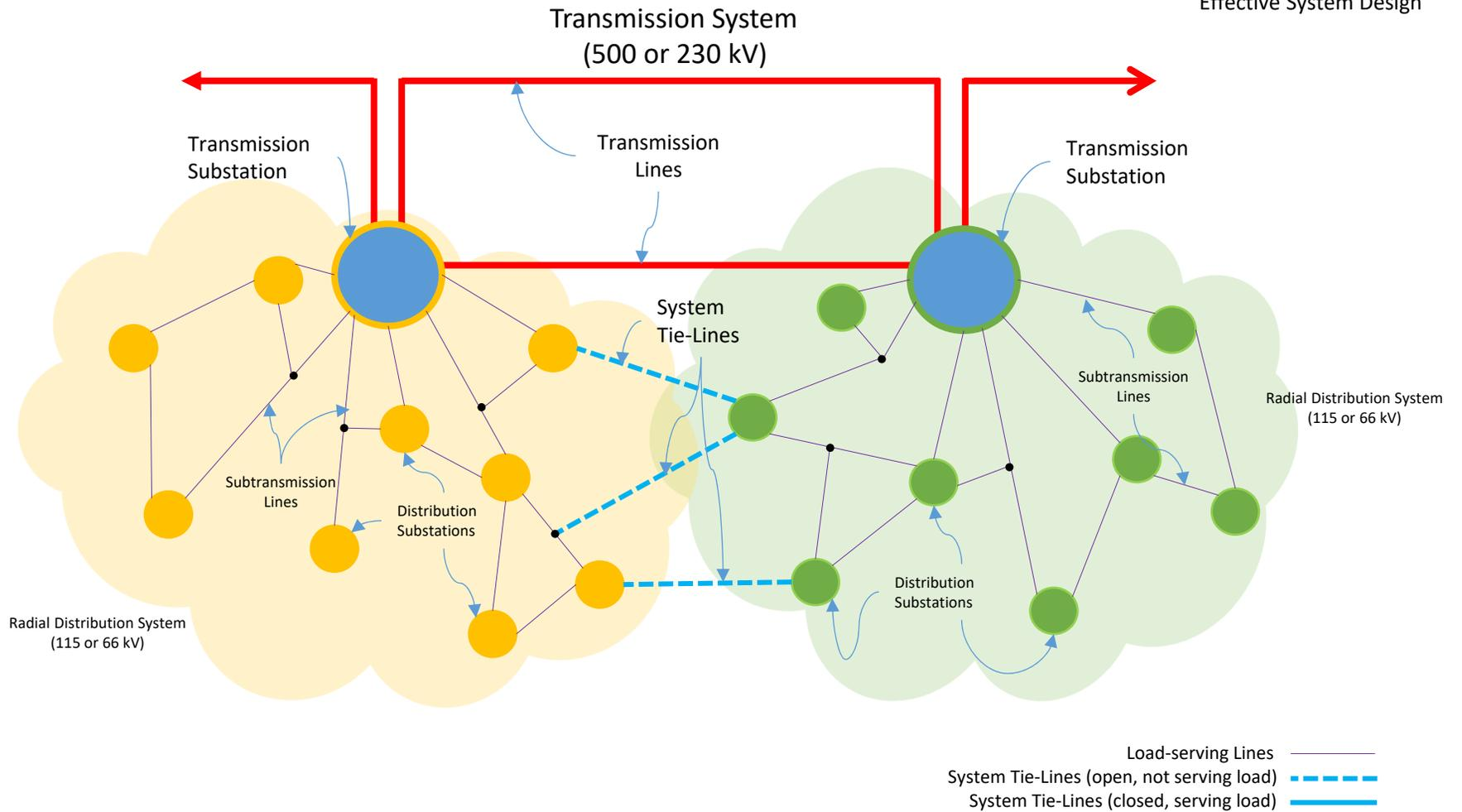
(2) Radial Distribution Systems with *effective* system tie-lines located “downstream” at the intersection of the two systems thus allowing for bi-directional transfer of substations without interfering with the reliable and safe operation of the remaining network following a transfer.
