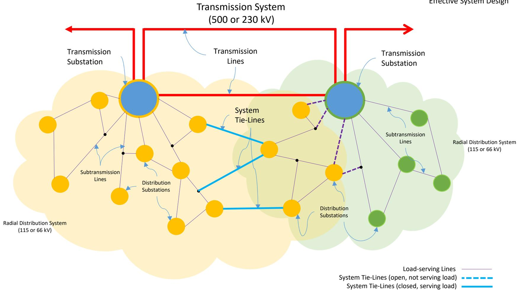
(2) Radial Distribution Systems with *effective* system tie-lines. Following an incident on the system to the right, the system on the left is able to effectively transfer significant load from the system on the right to provide relief and improving reliability and resiliency.
