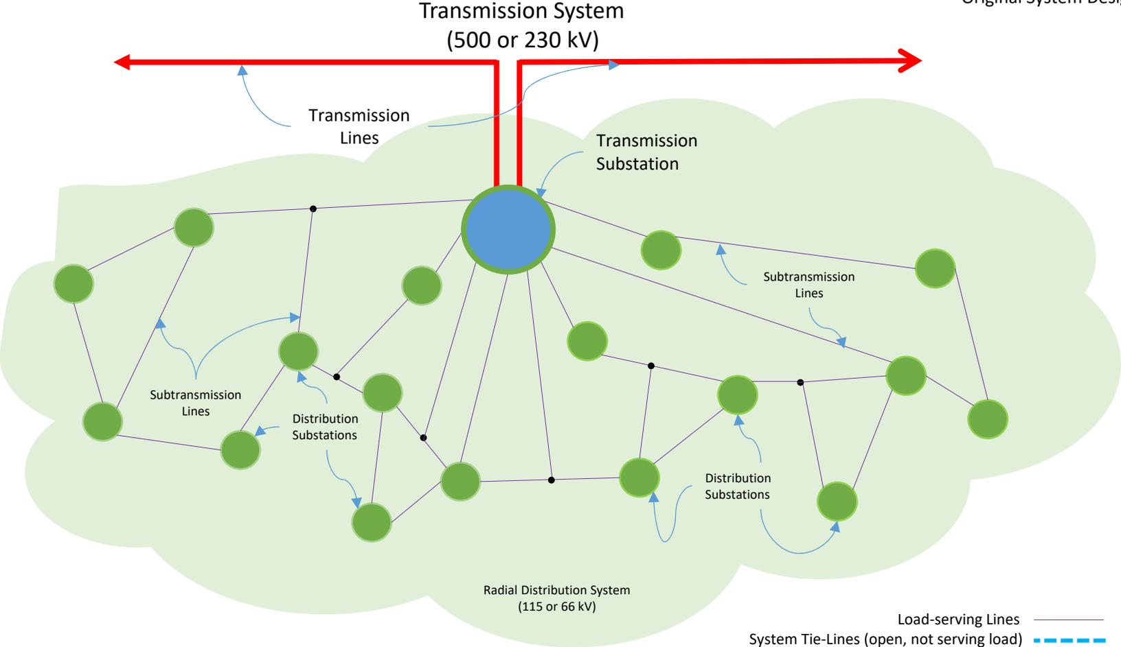
Radial Distribution System with no system tie-lines
