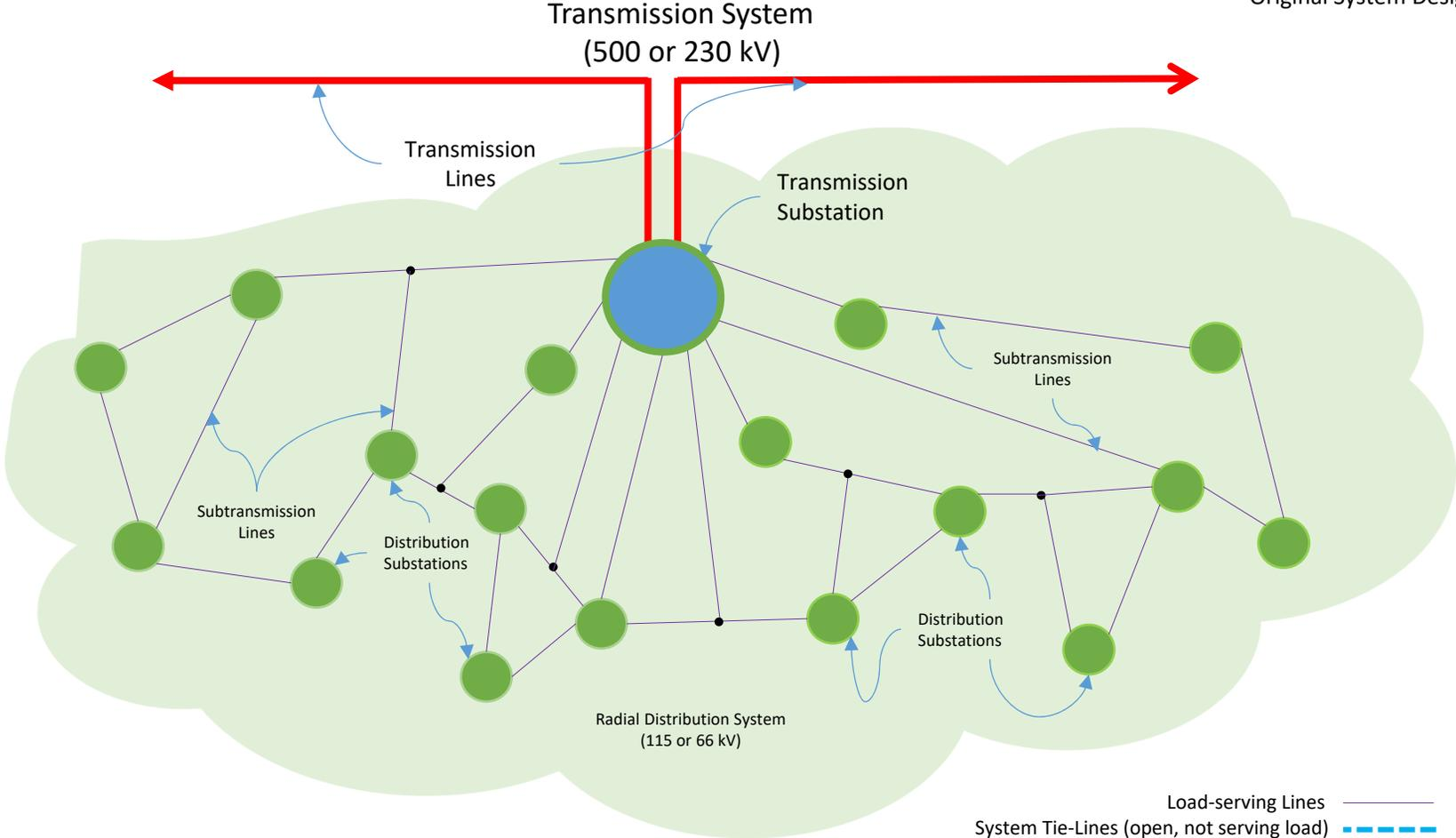
Radial Distribution System with no system tie-lines (same as Figure 1).
