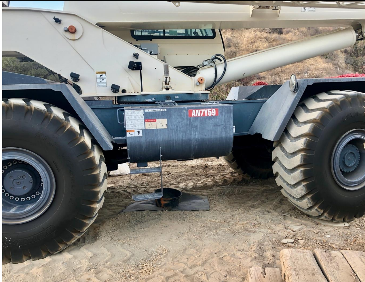
Photo 12 – Secondary containment under parked equipment.
