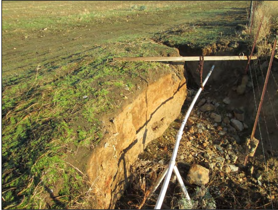
Photo 5. Concordia Yard paleontological field survey (conducted December 10, 2019): drainage channel exposure of middle to early Pleistocene-age very old axial-channel deposits (Qvoa), consisting primarily of sands and gravels. Larger cobbles and occasional boulders can be observed within the wash. Partially buried pipelines are exposed within the channel and near the top of the wash. View facing to the north.
