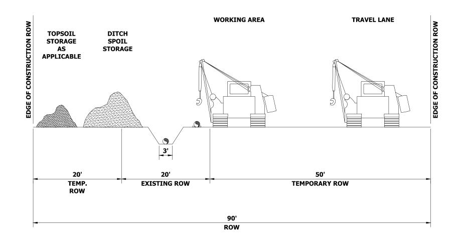
Typical Cross Country Construction Removal and Replacement of Line 1600 in Segments or as a Whole
