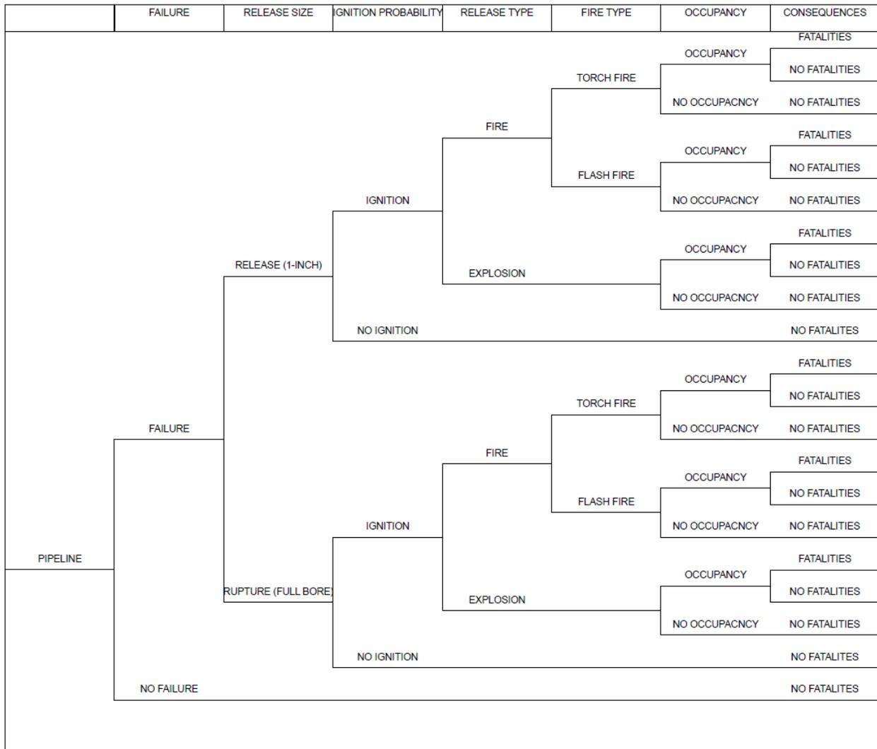
**Figure 8-1: Pipeline Event Release Tree**
