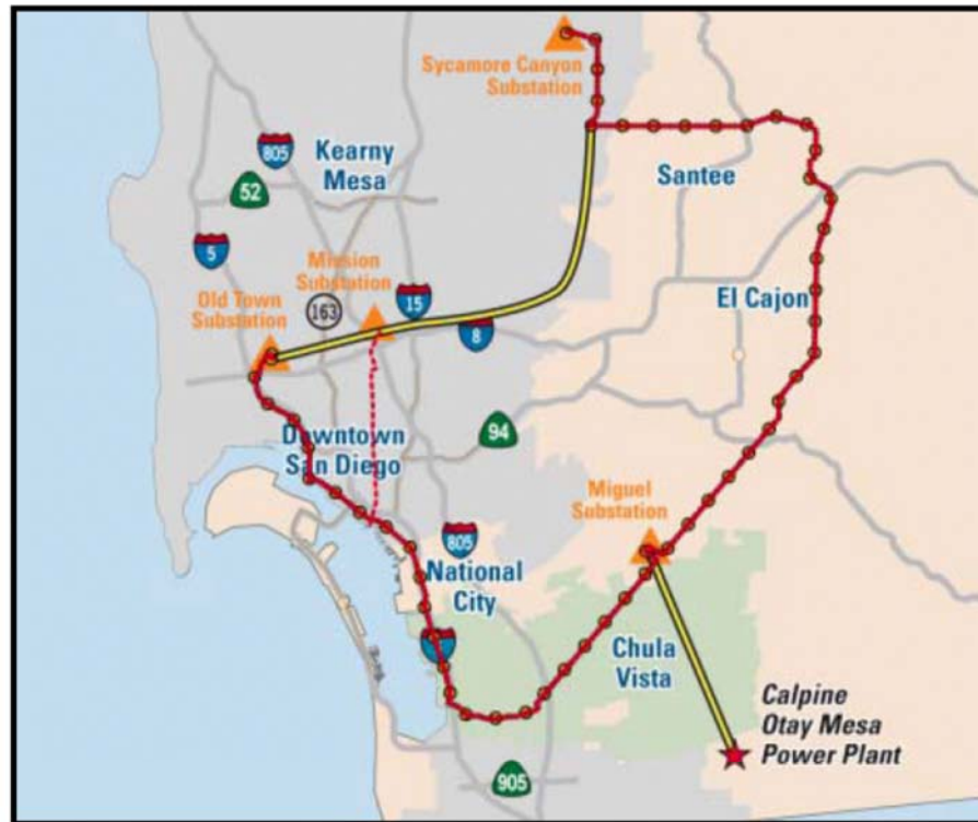
Figure 6: Electric Transmission Expansion for Otay Mesa
